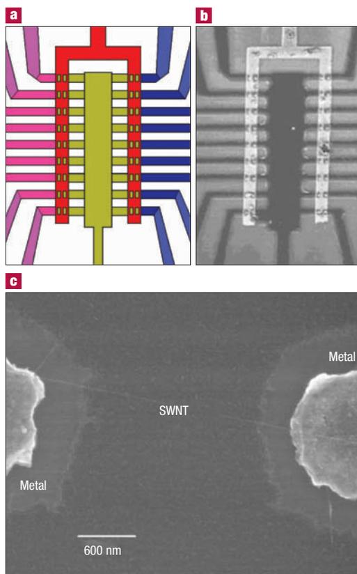
**Figure 1** Nanotube-based logic devices are being made with increasing sophistication; that shown here contains single-wall nanotubes (SWNTs) grown between contacts. **a**, A schematic and **b**, a scanning electron microscope image of a field-effect transistor. The nanotube is not visible as it is buried under the gate oxide and gate metal. **c**, A scanning electron microscope image of a single-wall nanotube linking two metal catalyst particles.
