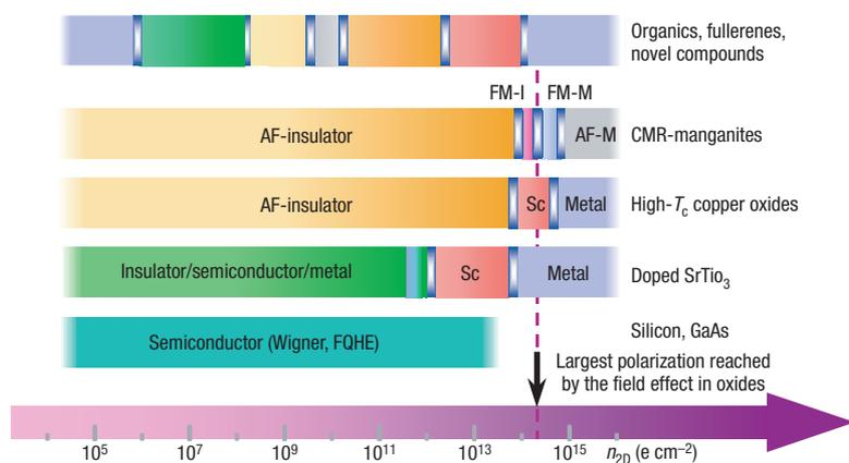
**Figure 2** Wide-ranging behaviours of correlated systems as a function of sheet charge density,  $n_{2D}$ . The data summarize results for many carbon-based systems and oxides at absolute zero temperature<sup>1</sup>. AM, antiferromagnetic; FM, ferromagnetic; I, insulator; M, metal; SC, superconductor; CMR, colossal magnetoresistive; FQHE, fractional quantum Hall effect.
